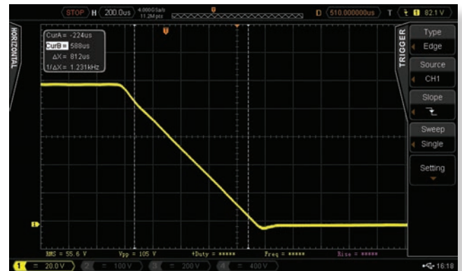
DC Voltage Ramp Down @ 100Vdc/ms programmed slew rate into 100Ω resistive load captured
